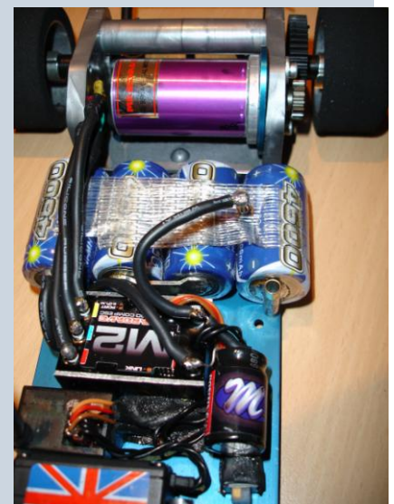
The Mardave brushless system, note smaller 400 size motor, speed controller also shown
